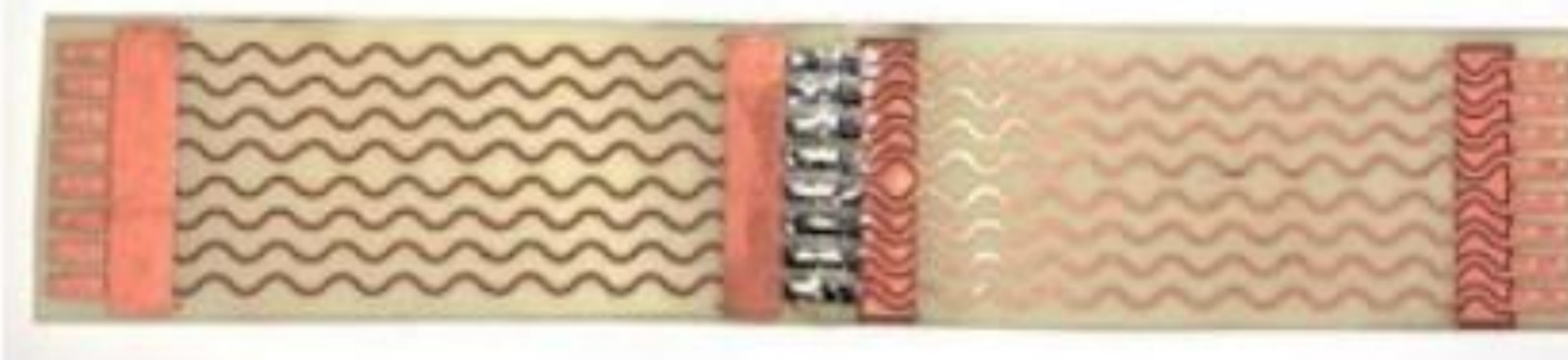
Eight parallel copper tracks connecting the contact pads at the left and right end of the FPC. Two FPC have been connected.
